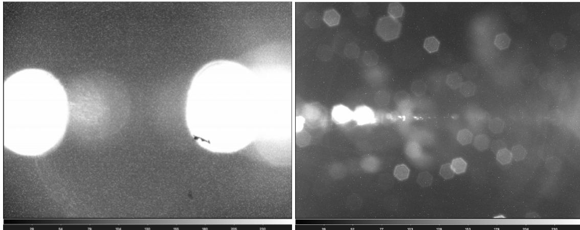
Figure 1. Example calibration images captured in-flight with the HRN camera (left) and TRN camera (right), showing significant scattered light reflected off of the spacecraft’s landing legs.
