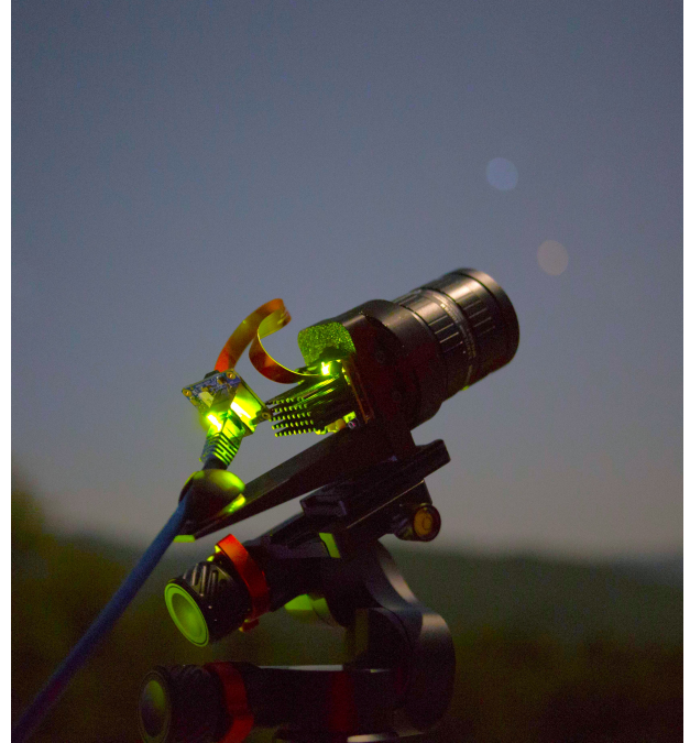
Figure 2. The first imaging field test was completed during which star field and Moon images were captured for camera calibration and initial horizon-based OPNAV techniques were tested.
