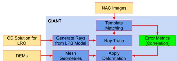
Figure 2. Flowchart of the NAC image comparison
