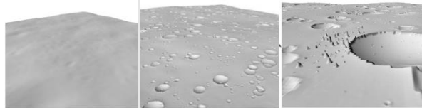
Figure 2. Left: Original, low resolution lunar terrain. Center: Upsampled lunar terrain with crater features. Right: Crater with procedural rock hazards.
